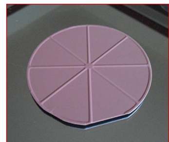
Compliant Spoke Features Pin Chuck and Handler Arm
